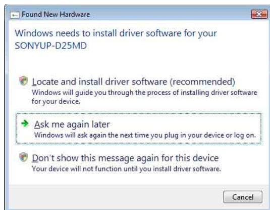
If the “Device driver software was not successfully installed” message appears and the [Found New Hardware] dialog box does not appear, try disconnecting and connecting the USB cable again. If the [Found New Hardware] dialog box still does not appear, perform the steps described below, with the printer for which the printer driver is to be installed turned on and connected to the computer. (Any other USB printers or previously installed printers should not be connected at this time.)
